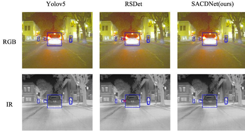
Fig. 5. Visual comparison under extreme nighttime conditions with severe vehicle taillight glare. From left to right: YOLOv5, RSDet, and SACDNet(ours). Our proposed method successfully suppresses the extreme glare to accurately bound the vehicle, while also detecting the pedestrian hidden in the dark background on the right.
