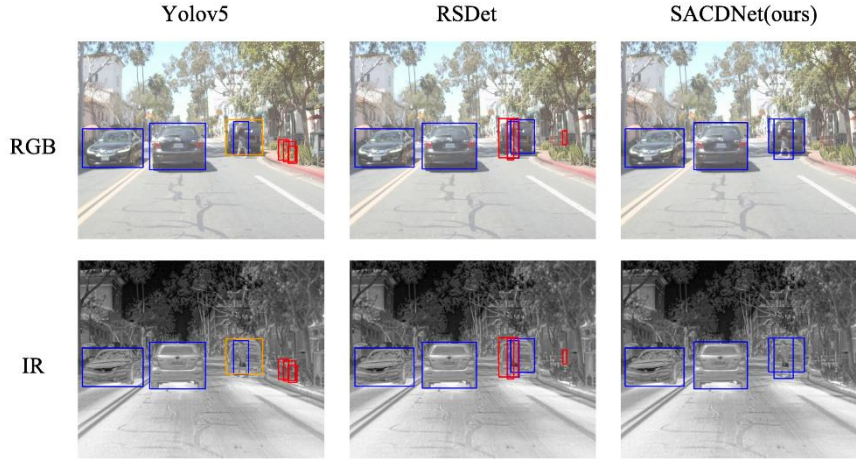
Fig. 6. Visual comparison in scenes with severe instance occlusion. From left to right: YOLOv5, RSDet, and SACDNet(ours). Our method accurately resolves overlapping targets without generating ghost predictions.
