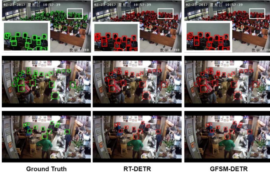
Fig. 5. Visualization of detection results. Green bounding boxes indicate ground truth targets, while red bounding boxes represent the model’s detections. The white bounding boxes indicate the areas we need to magnify for detailed observation.
