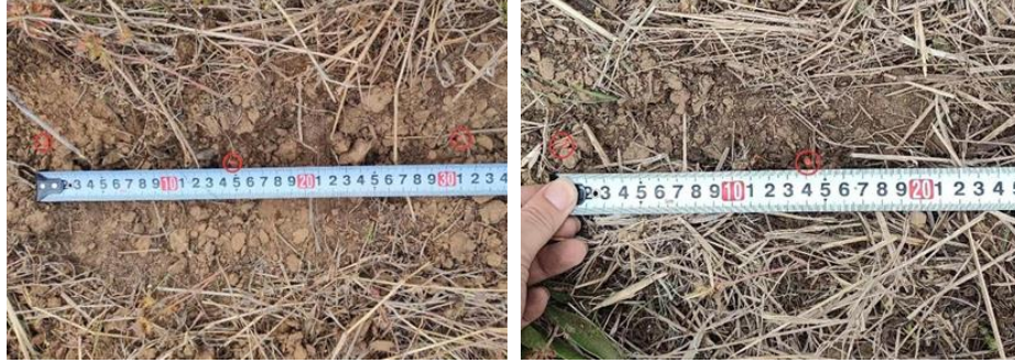
Fig. 7. The red circles in the figure indicate corn seeds sown by the planter. Seed spacing is measured using a ruler.
