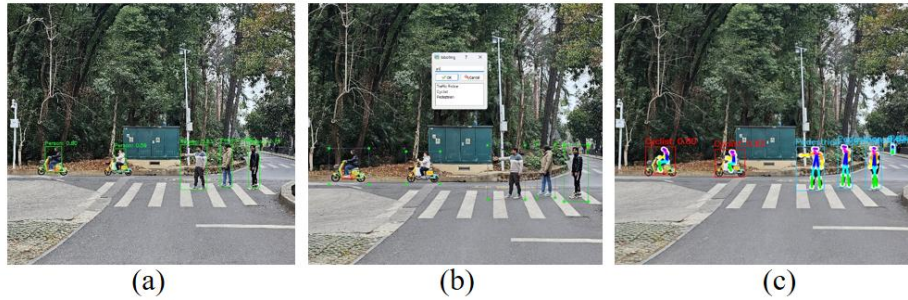
Fig. 5: Comparative analysis of detection performance between the official YOLOv8 baseline model (a), Data annotation process (b) and our customretrained model on proposed dataset video, where pedestrian, cyclist and traffic police are different class, featuring enhanced spatial feature extraction using Openpose (c).
