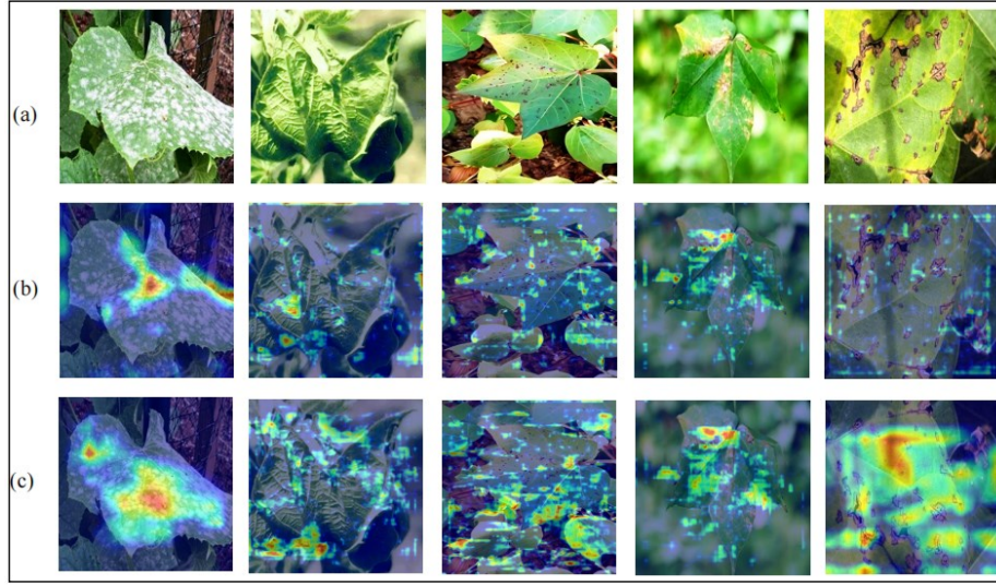
Fig. 6. Comparison chart of thermal effects on Cotton Pest Detect Dataset, where (a) is the original image, (b) is the YOLOv8n detection thermal map, and (c) is the SDRM-YOLO detection thermal map
