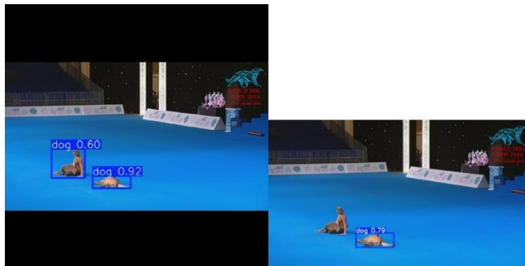
Fig. 2. YOLO detection result(left image is resized to 512 \times 512 , right image is 1280 \times 720 ) [5]
