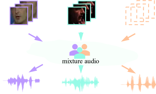
Fig. 1. Diagram of our overall AV-MSS framework under the missing visual cue condition. This figure depicts the 3-mix scenario with two available visual cues.
