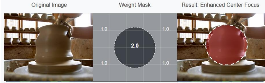
Fig. 4. Center Region Weight Mask (2.0 Center, 1.0 Periphery).
