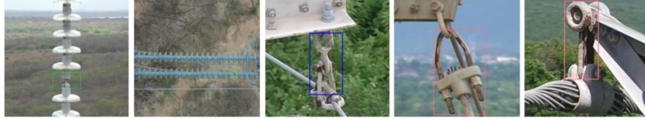
Fig. 2. Example of annotation, in which different color of rectangular boxes represent different fault types.
