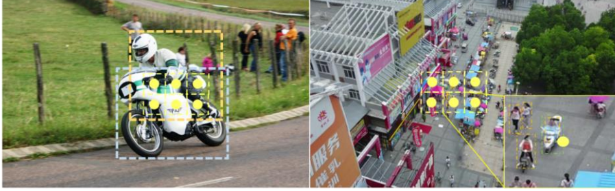
Fig. 3. An illustration of ambiguous anchor points in object detection. Yellow dots show some of the ambiguous anchors in two sample images. The large object (left) is due to large area, resulting in overlap. And the small objects (right) are assigned to the same anchor due to its small area.
