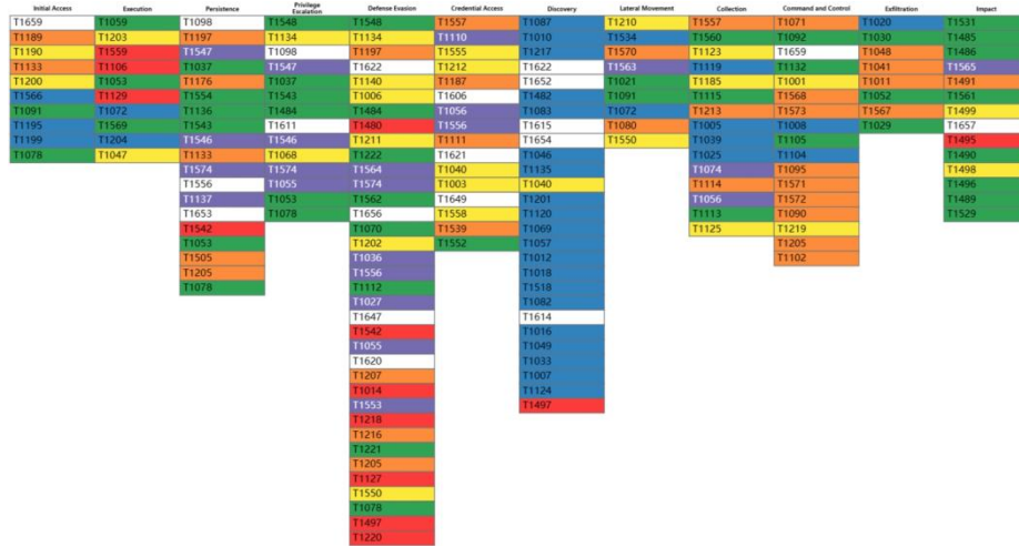
Fig. 3. ATT&CK Navigator Organized with Difficulty of Exploitation. Blue- not really exploitable; green- the easiest techniques to exploit; yellow- need some sort of tool; orange- requires some level of infrastructure to setup; red- the most advanced techniques which require an in-depth understanding of the OS or custom DLL/EXE files for exploitation; purple- high level techniques which include sub-techniques of varying levels; and white - not labeled due to version of ATT&CK matrix.
